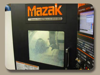
The DSO lathe department consists of 7 CNC lathes with turning capacity of 28.4". Our lathe lineup consists of four Mori Seki's, one Nakamura,one Hwacheon, and one Mazak QTN450, along with three manual lathes for secondary or fixturing operations.
